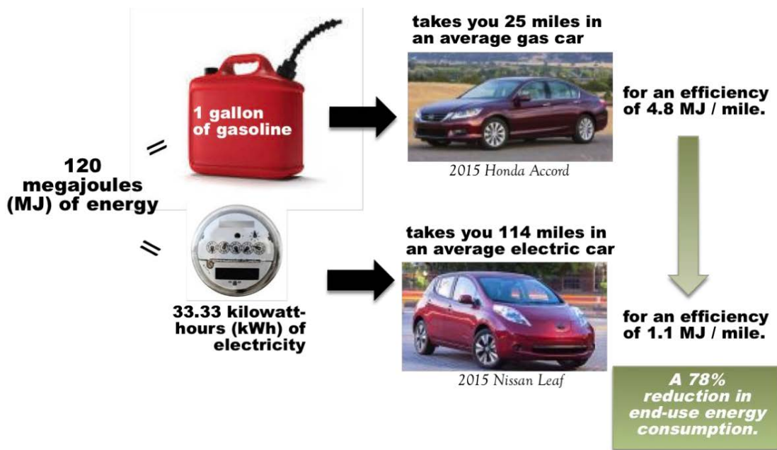
Figure 2: Illustration of Relative Efficiency of an EV and a Gasoline-Fueled Vehicle 19
