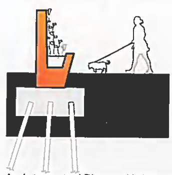
An Integrated Planter Unit in a single mold provides cost and installation efficiencies compared to attached discrete planting elements
