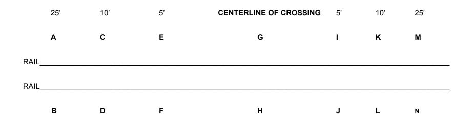
NOTE: All field markouts shall be accomplished using a paint or keel marker, chisel cuts are prohibited on the rail.
