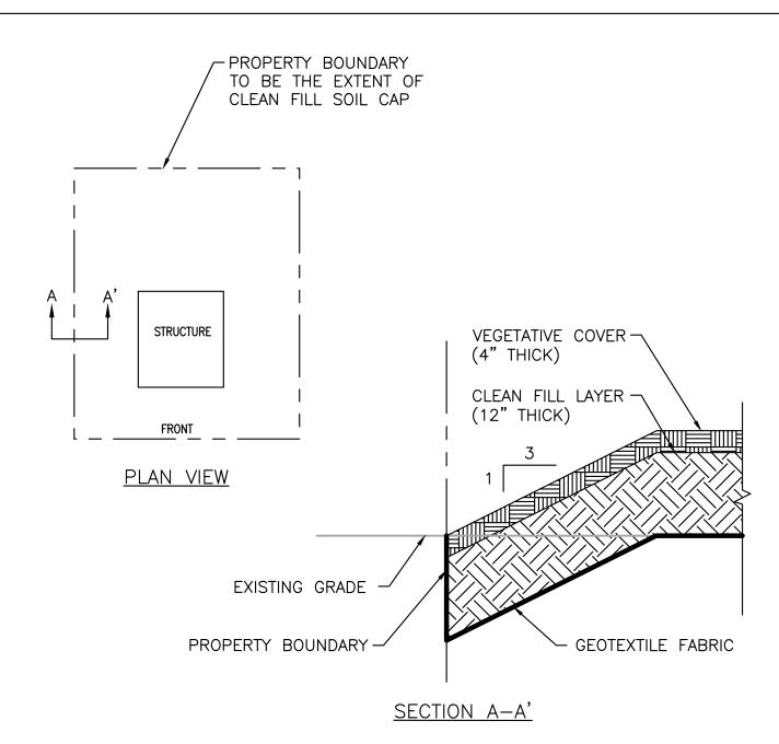
NOTE: CUT SOIL TO BE USED AS BACKFILL TO GRADE SITE PRIOR TO APPLYING CLEAN FILL SOIL CAP.
