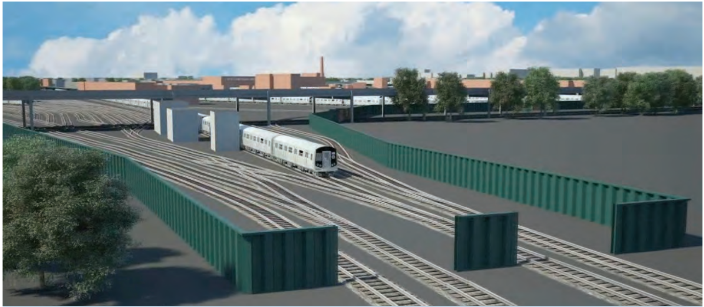
Rendered view of Coney Island Yard Sheet Pile Flood Wall Concept
