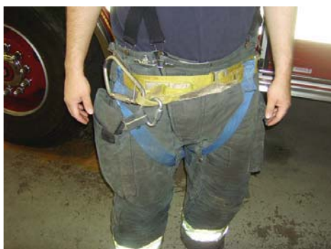
Figure C-10. A Class II Harness is secured around the waist and thighs.
