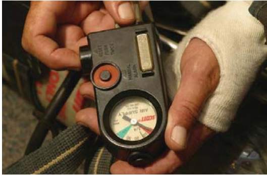
Figure C-12. Various types of PASS Devices are available. Including those that are integrated with SCBA
