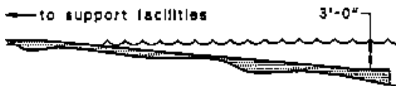
Figure 7.6c Ramp Into Water
