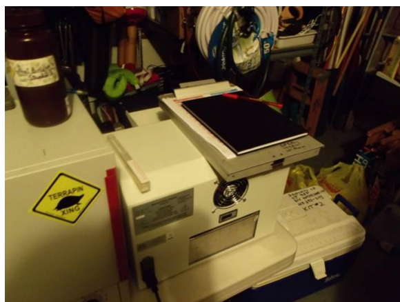
Figure 5. Lab station. Incubator, IDEXX sealer, and cooler.
