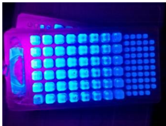
Figure 7. IDEXX Quanti-Tray 2000. IDEXX Quanti-Tray 2000 containing Enterococcus indicated by many fluorescing wells of a sample collected from Beachwood Beach West on July 29, 2011.
