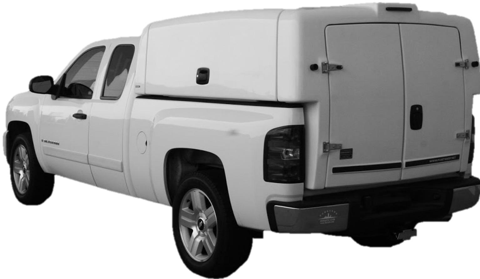
Likely just an insulated box, but the refrigeration unit may be inside. Likely electric - check for connections.
