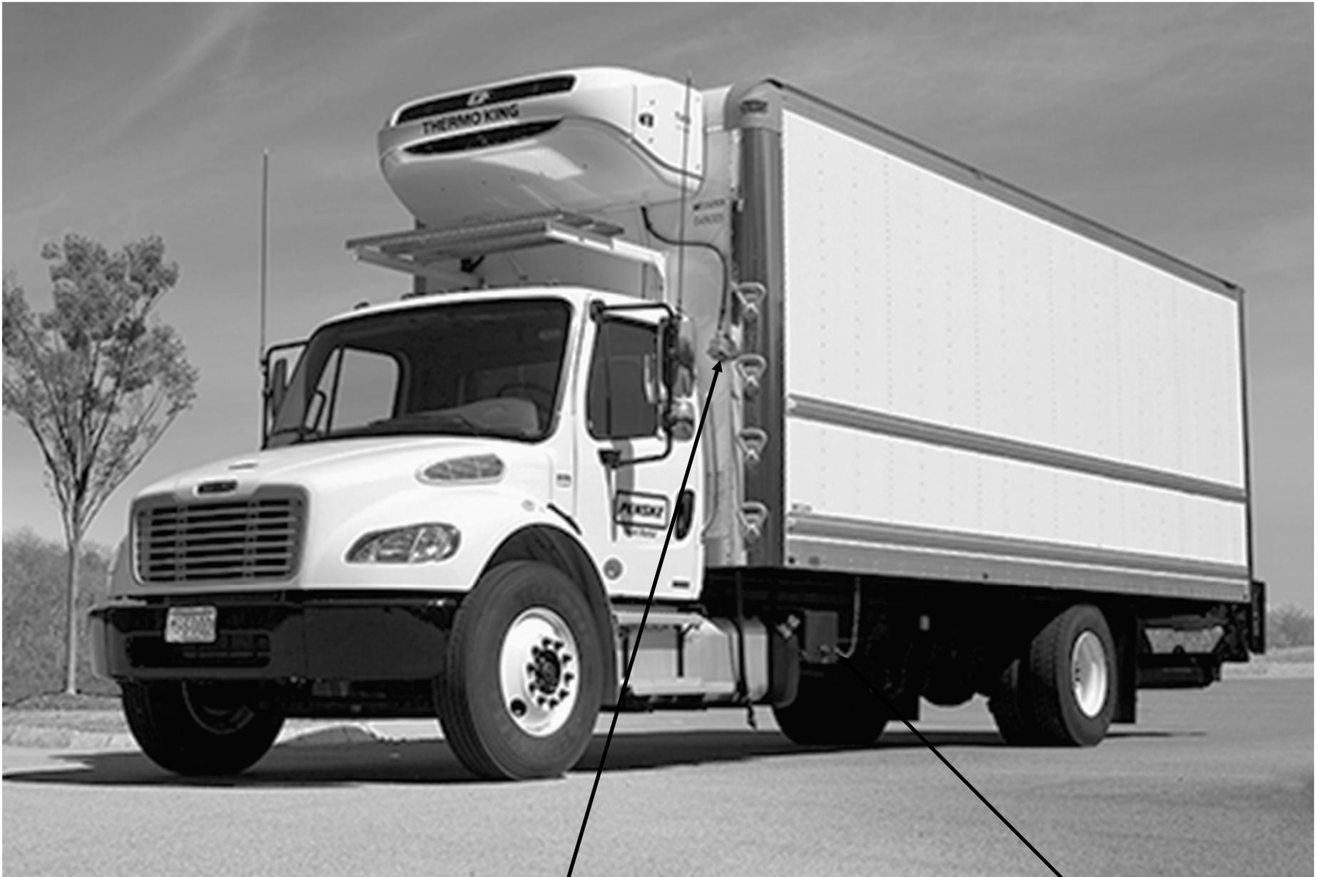
Note shore-power connection and frame-mounted tank
