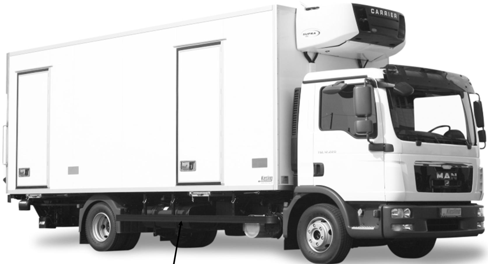
Guard rails are an indicator for TRU tanks.
