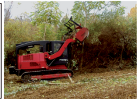
Forestry Mower— Reducing brush to Mulch
