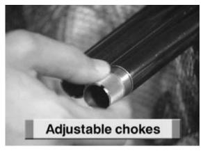
The muzzle end of a shotgun barrel has a choke, which is used to control the spread of shot downrange. The choke is much like the nozzle on a garden hose. A full choke constricts the water into a tight stream. A cylinder choke opens the spray up to shoot a wider cone.
