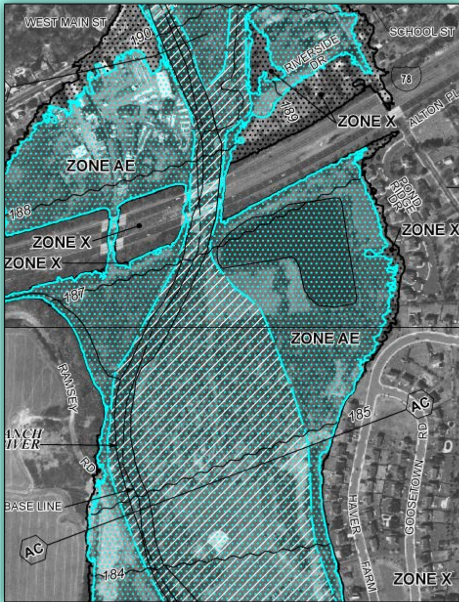
Figure 4.15: FEMA Map Showing a Fluvially Controlled Flood Hazard Area
