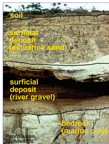
Figure 1. Examples of soil, surficial deposits, and bedrock in New Jersey. In northern New Jersey (left, photo by S. Stanford), bedrock is consolidated sedimentary, igneous, and metamorphic rock. In southern New Jersey (right, photo by J. P. Owens, USGS), bedrock includes unconsolidated marine deposits.
