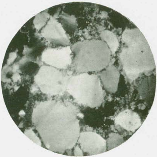
A. Thin section, crossed nicols, X 50. Specimen from point near Pohatcong Creek, one and a half miles northeast of Bloomsbury. Dolomite replacing quartz grains in Lower Kittatinny near contact with Hardyston.
