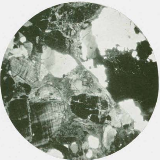
B. Thin section, crossed nicols, X 18. Hardyston specimen from southwest nose of Scotts Mountain, showing quartz and microcline grains cemented by iron oxide.
