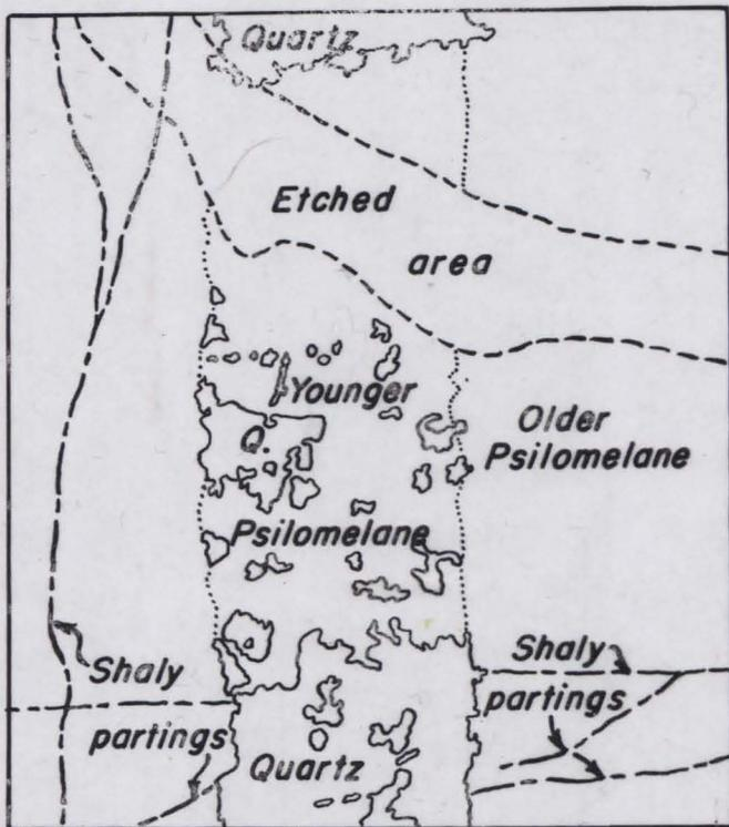
PLATE II—Photomicrograph of an etched polished surface of psilomelane, quartz and shale. The groundmass of psilomelane and unreplaced shale is cut by a inlet of quartz which is partly replaced by a later generation of psilomelane. Plane light, 120X.
