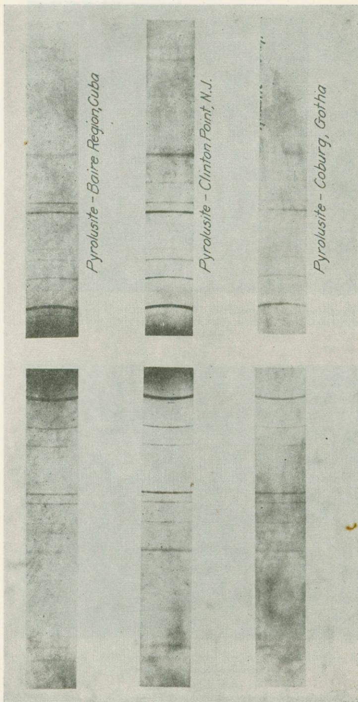
PLATE IV — X-ray powder diffraction patterns of pyrolusite taken in a Debye camera of radius 57.3. Unfiltered iron radiation.
