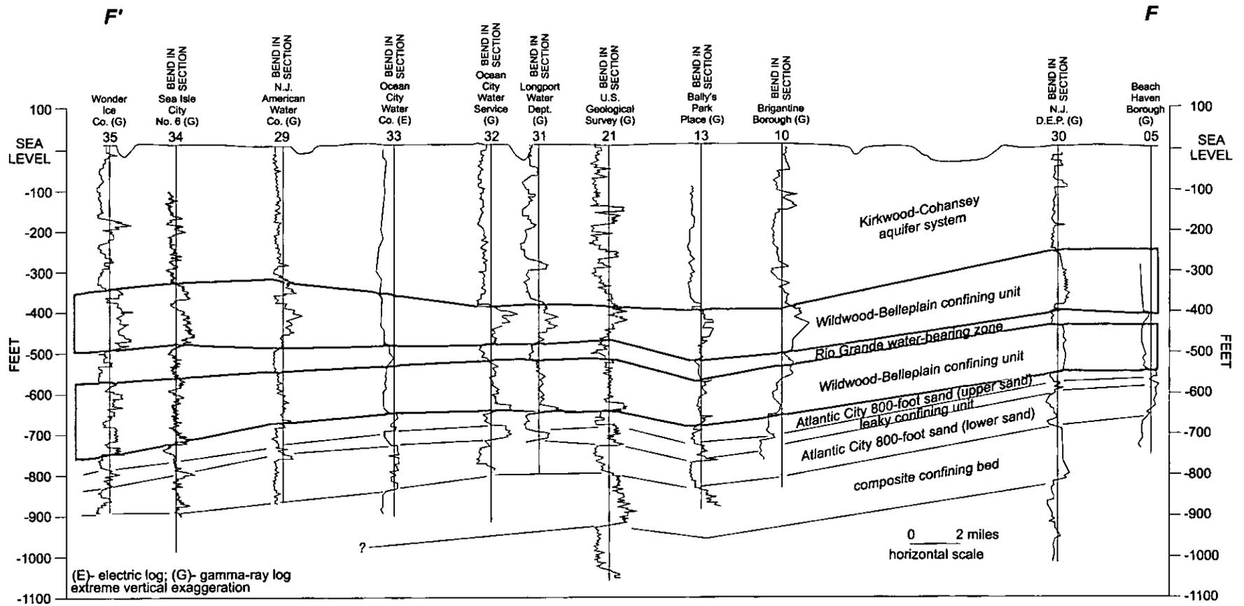
Figure 12.-- Cross-section F'-F.
