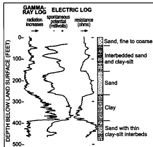
Figure 6.— Idealized borehole geophysical responses to lithology.
