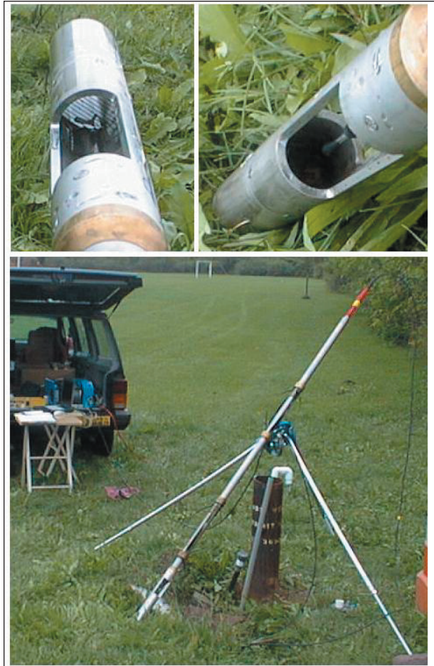
Figure 1b. Photographs of the HPFM before deployment in a well. The HPFM is resting against the tripod/pulley assembly in the bottom photograph. The photo on the upper left shows the heating grid in the tool aperture. The top right photo shows the upper thermistor in the tool aperture.
