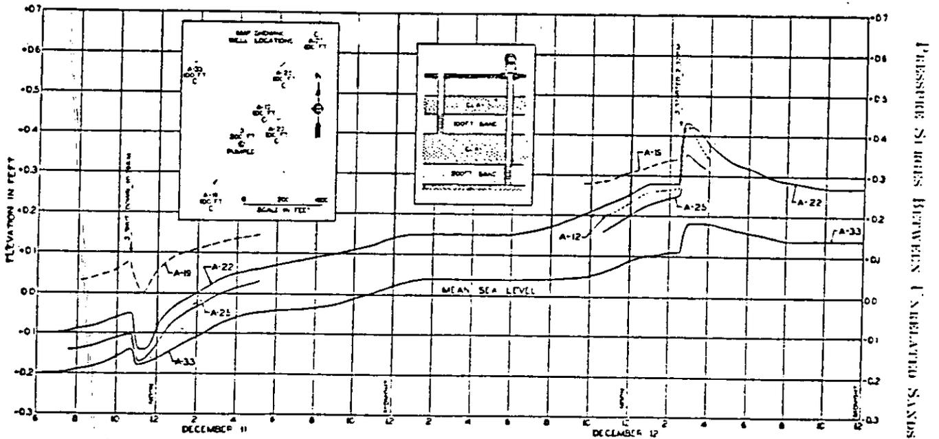
—Effect of starting and stopping a well to the 200-foot sand, at the Atlantic City Water Works, on water levels in wells to the 100-foot sand, with a map of the wells observed.
