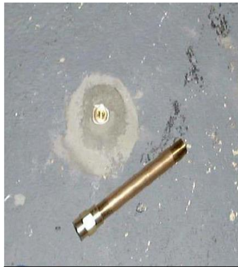
Figure 6-2 Grouted Hole with Vapor Probe (DiGiulio et al. 2005)
