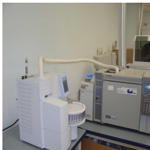
Figure 6-4 Autosampler GC/MS for TO-17 analysis (courtesy of Severn Trent Laboratories)
