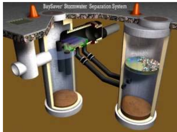
Figure 1. BaySaver Separation System
