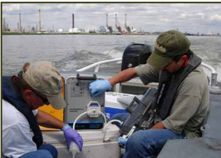
DRBC Geologist Greg Cavallo (right) holds the Niskin sampler and operates a portable pump while Modeling, Monitoring & Assessment Branch Manager Dr. Tom Fikslin holds a filter and fills a sample bottle. This technique being used during a special copper survey on the Delaware River results in very low contamination of the sample by other metal sources. (Photo by DRBC)
