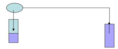
Grab sampling using peristaltic pump, teflon sampling tubing, 2L bottles
