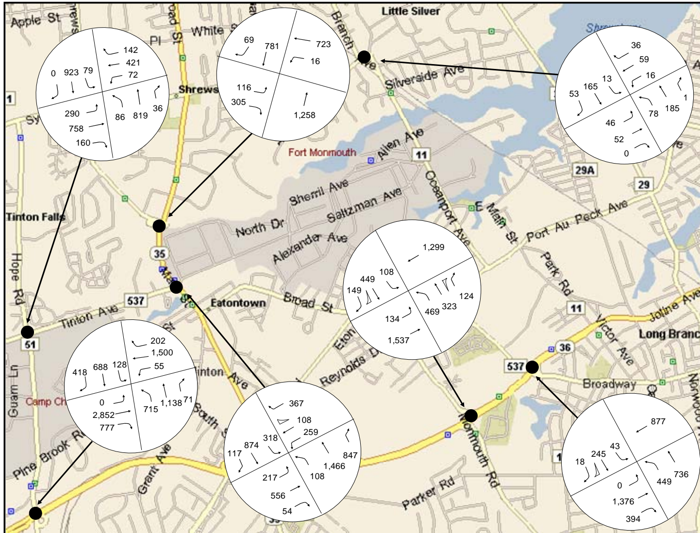
Figure 3-4: 2028 Build-Out PM Peak Hour Traffic Volumes
