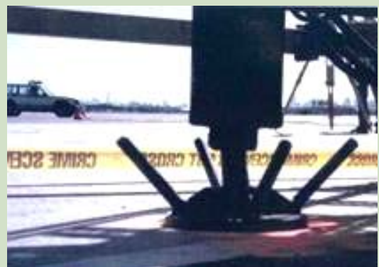
Close-up of central stabilizer support pad in down position
