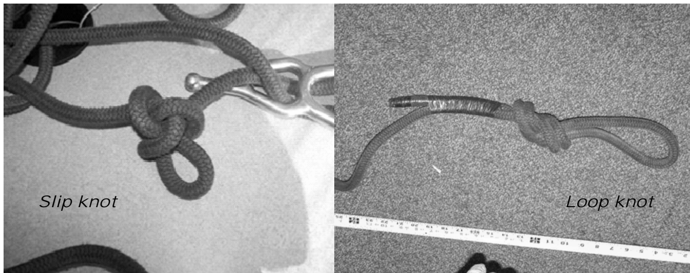
FIGURE 2. Lifeline: Controlled descent device or Fisk, along with slip knot and loop knot at each end of the lifeline.
