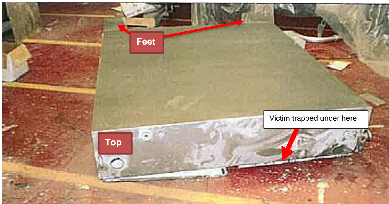
FIGURE 2. Incident scene; cabinet fell forward crushing the victim underneath.
