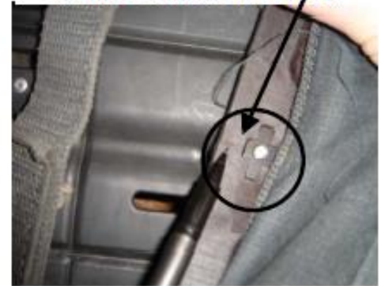
Crack At Lumbar Support Caused Separation Failure
