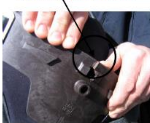
Crack From Pulling & Dragging
