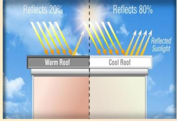
A schematic of sunlight reflecting from a traditional roof and a cool roof. Four times the amount of sunlight is reflected from a cool roof.
