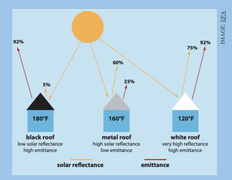
Illustration of solar reflectance and thermal emittance shows how they vary with color and material. White roofs reflects the most amount of sun, and although both white roofs and black roofs have high emittance, white roofs keep much cooler overall.
