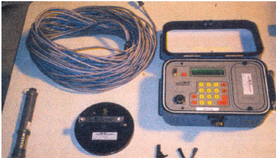
Figure A. Components of the GECOR 6 Corrosion Rate Meter
