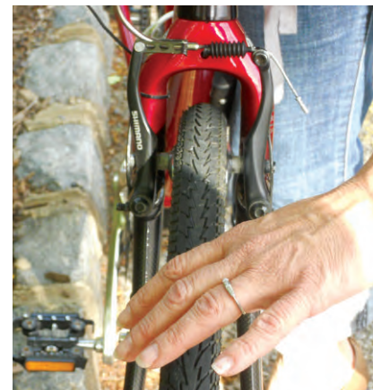
Checking Tire for Damage
