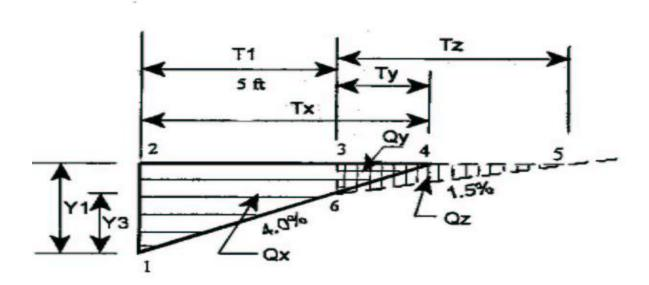
Initially, a depth is assumed (y1). Qx,Qy and Qz are then calculated using the above equation. The flow contained in the composite section (Qt) is equal to Qx + Qz - Qy. This process is repeated until Qt = Q (actual flow in the gutter). T (actual spread width) is equal to Tx+Tz-Ty.
