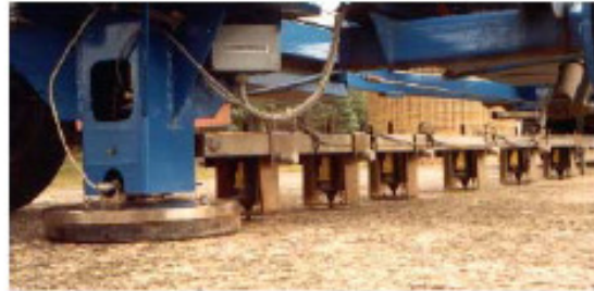
Figure 9.22: FWD Impulse Loading Mechanism (foreground) and Sensors (background)
