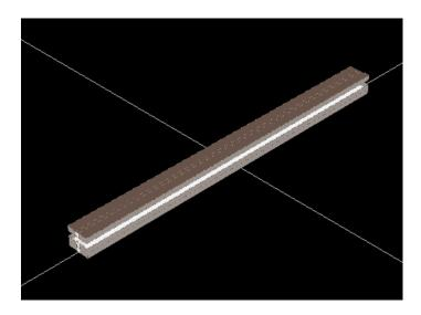
Note: The middle floors, since they thermally equivalent, are simulated as a single floor, and theresults are multiplied by 2 to represent the energy consumption of the 2 middle floors.
