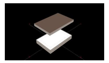
Note: The middle floors, since they thermally equivalent, are simulated as a single floor, and theresults are multiplied by 8 to represent the energy consumption of the eight middle floors.
