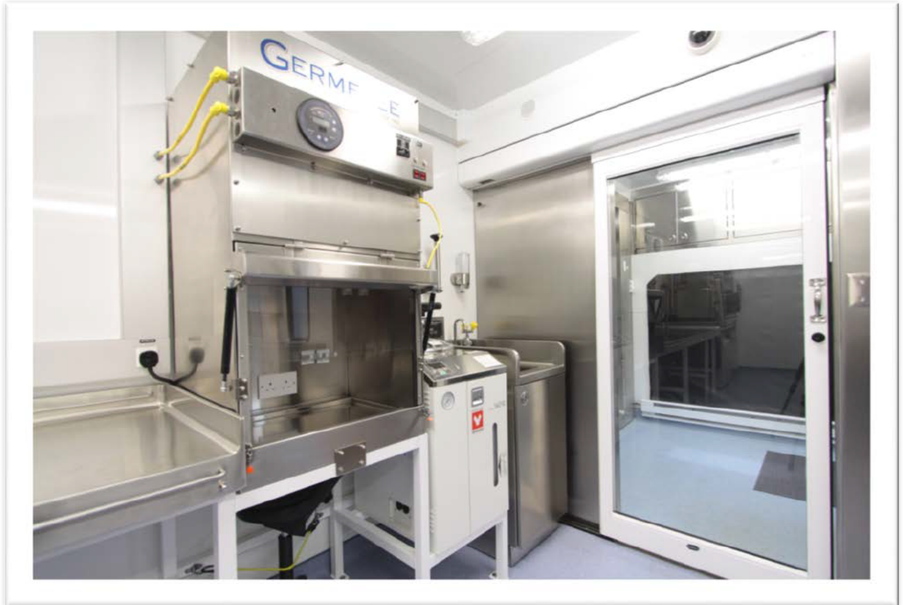
Class II Type A2 Biological Safety Cabinet (PCR/Media Prep hood) and top-load autoclave at lab exit (For display only)
