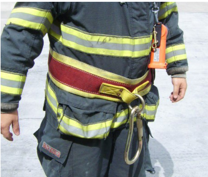
Figure C-11. A Class I harness is secured only around the waist. John Lewis.
