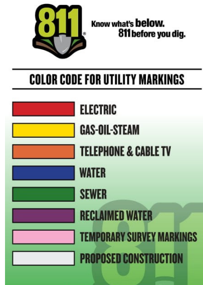
Figure D-16 State Law mandates that contractors and the general public call for a Mark-Out at least 3 business days prior to planned excavation.. NJ One Call.
