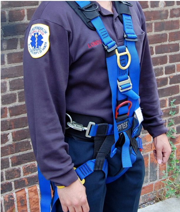
Figure C-13. A Class III harness is secured around the waist, buttocks and shoulders. Robert Moran.
