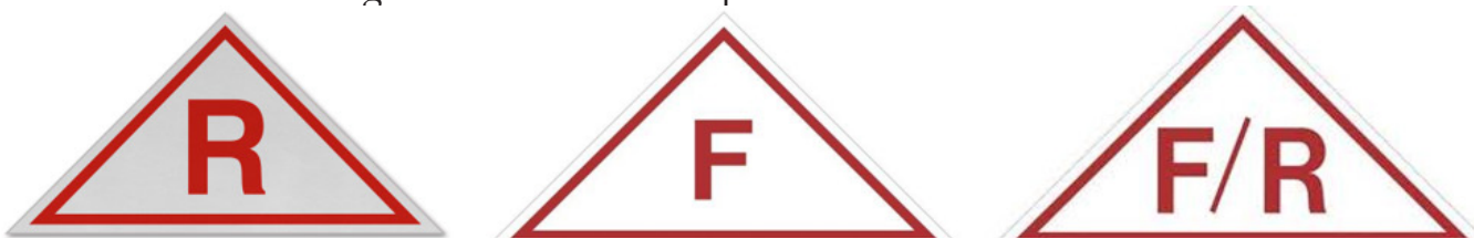
Figure C-28. Truss Roof Identifiers for Roof (R), Floor (F) and Floor /Roof (F/R). NJDFS UFC.
