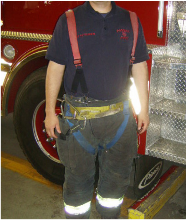
Figure C-12. A Class II Harness is secured around the waist and thighs. John Lewis.
