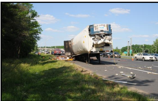
Figure 1 - Front of trailer damage to Refrigeration Unit
