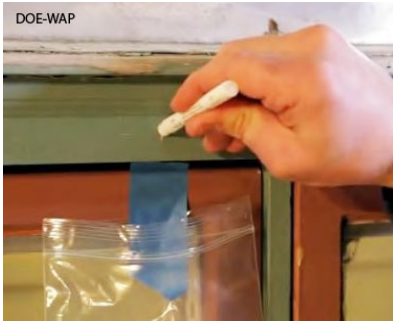
First, crush the capsule and shake it to mix ingredients. Then swab the sample for 30 seconds.
