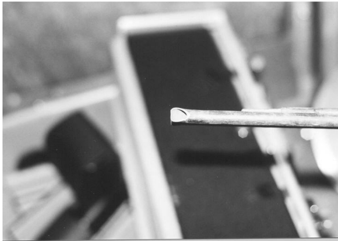
Figure 2-2. Properly Constructed Type S Pitot Tube.
