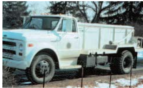
Distribution vehicle, equipped with a four-compartment tank, pony motor and pump, was used from mid-1950 to mid-1970.
