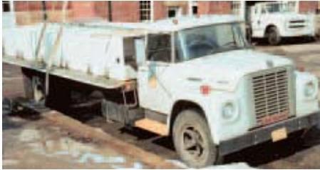
Upgraded stocking vehicles such as this, used from mid-1960 to late 1980, were equipped with a 16-compartment wooden tank and a roots blower system for aeration.
