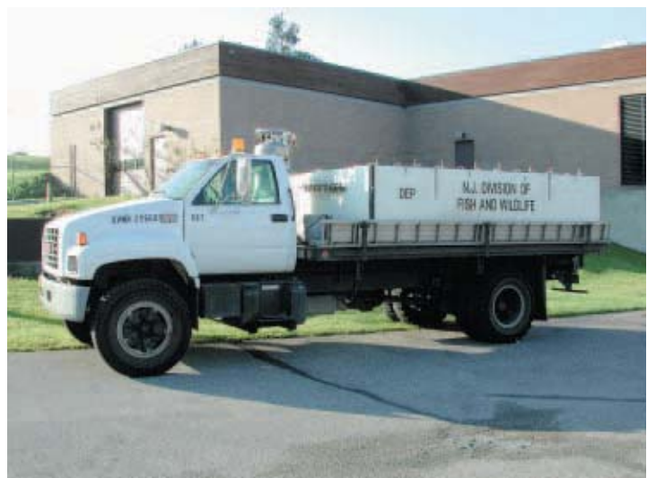
One of eight diesel-powered trucks equipped with oxygen injection systems (mid-1990 to present).
