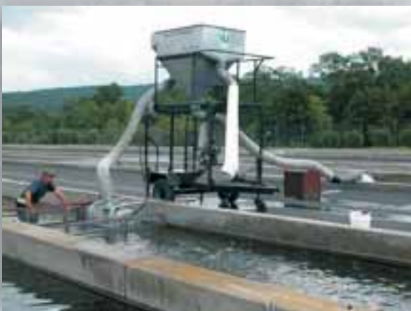
This fish pump is used to safely move fish into trucks in preparation for stocking.
