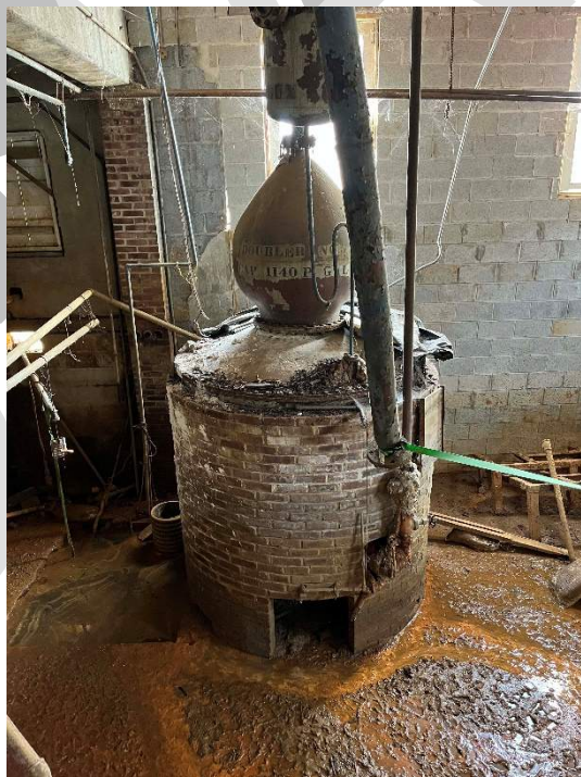
Photo 38. Detail view of original brick pot still used for applejack distilling, located inside the Still House, camera facing west (November 17, 2023).
