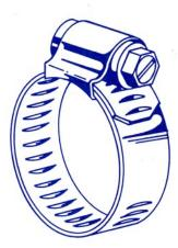
Fig. 8 – Hose clamps, regardless of style used, should be all stainless steel.
