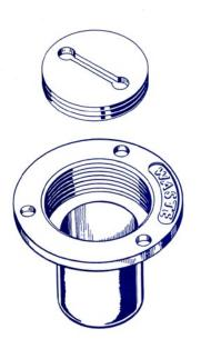
The Federal standard for a deck fitting for pumpout is 1 ½" inside diameter pipe thread. Most pumpout stations have adapters that will fit boats not so equipped.
