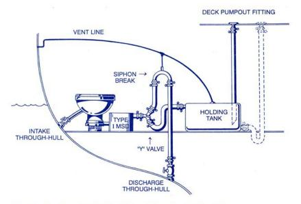
Fig. 4 – Overboard discharge option before the holding tank.
