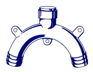
Fig. 11 – Siphon breaks have a one-way valve at the top to allow air to enter the line.
