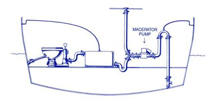
Fig. 13 – Macerator pumps can be used to break up and pump wastes from holding tanks for discharge in the ocean beyond the three mile limit.
