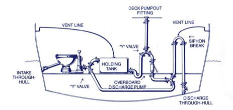
Fig. 3 – Overboard discharge options both before and after the holding tank.
