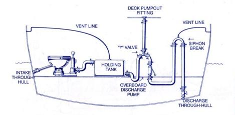
Fig. 2 – Overboard discharge option after the holding tank.
