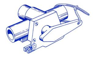
Fig. 12 – When operating within the three mile offshore limit, "Y" valves must be secured to prevent the discharge of sewage overboard. Acceptable methods of securing the valve include using a padlock or nonreusable wire tie wrap, or by removal of the valve handle.
