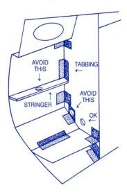
Fig. 14 – When running piping, avoid cutting into stringers or tabbing that support the hull so that structural integrity is not compromised.
