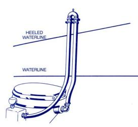
Fig. 10 – Siphon break fittings must be located above the maximum heeled waterline if they are to operate effectively.
