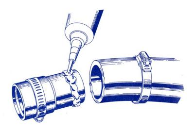
Fig. 15 – If a sealant is used when fitting a hose, it should be applied to the outer surface of the adaptor only.
