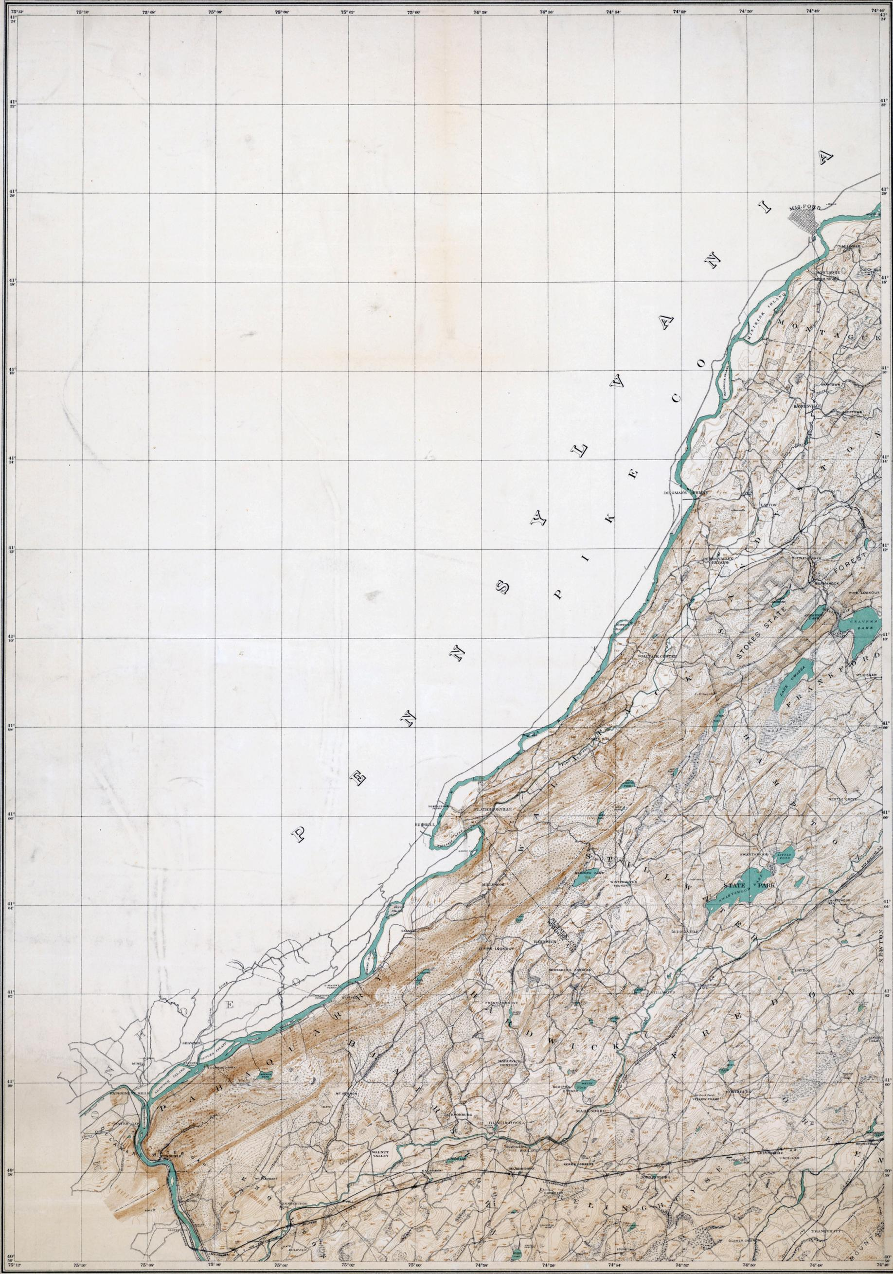
NOTE: The contour lines are level lines drawn on the earth's surface. All points through which they pass are of the same level and their height above sea level is shown by the figure on the line. The rise or fall from any line to the next is the figure will show on both. Figures not on any line show the actual elevation of the surface at a point indicated by a small cross.
