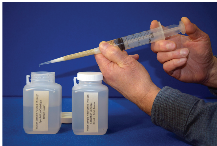
Figure 4. Use of arsenic speciation cartridge. Photo by Z. Allen-Lafayette
