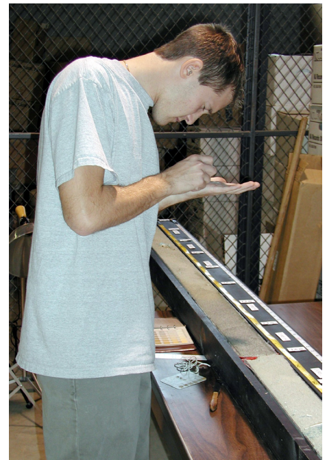
Figure 5. Geologist noting geologic characteristics of an extracted Vibracore (split and placed in black tray). After completing a geologic description of the core it is photographed and sampled for laboratory analysis.
