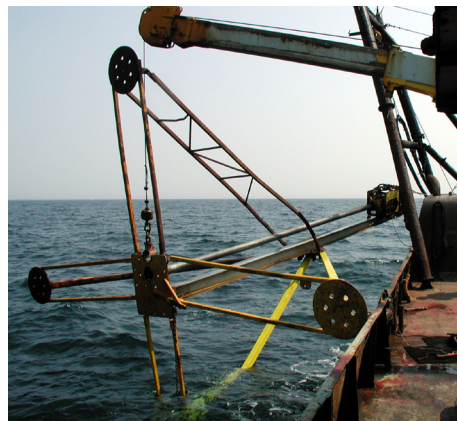
Figure 4. Vibracore rig being deployed off the side of a boat. The four-legged base (foreground) is rotated to sit on the ocean bottom. The core barrel is vibrated up to 20 feet into the sediments.
