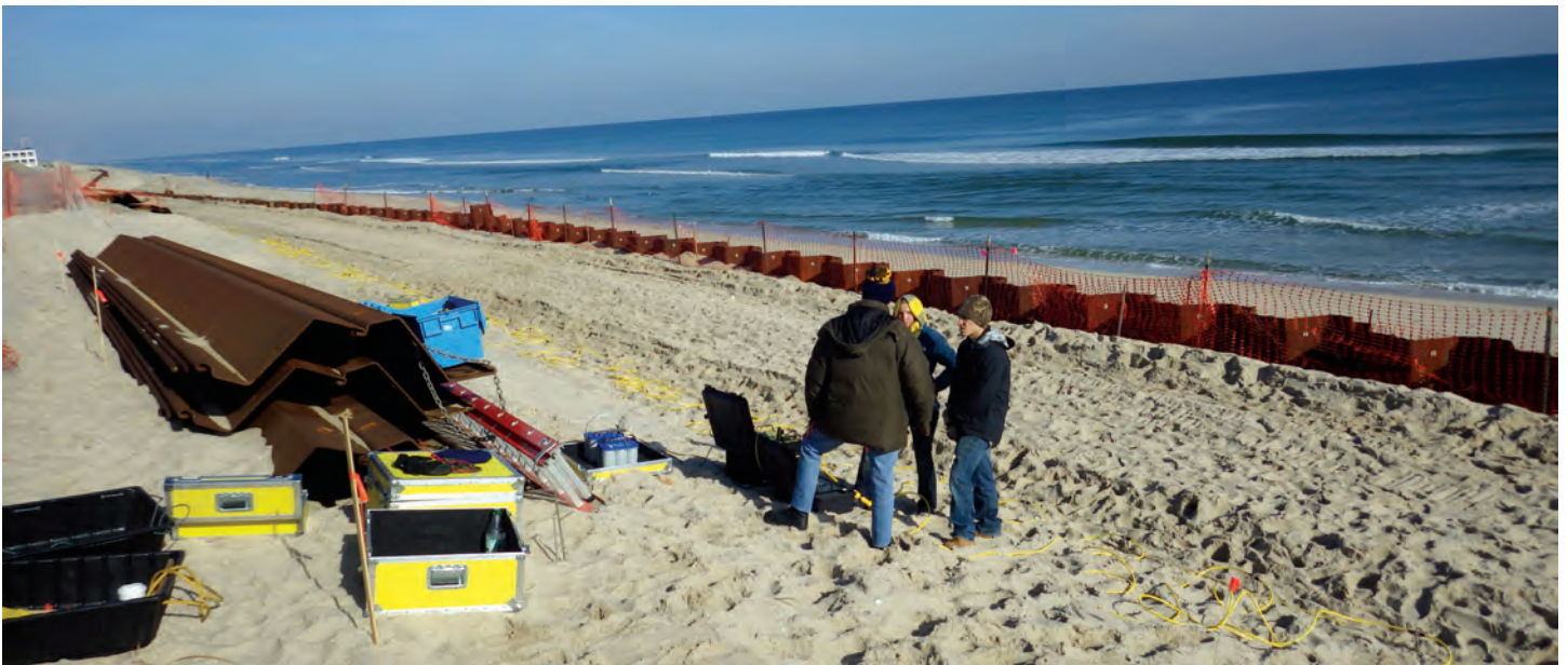
Figure 2. Set-up of resistivity array along the beach. NJGWS staffers (left to right) are Mark Godfrey, Michelle Kuhn and Mike Castelli. The seawall is on the right, additional steel pilings are on the left. Photo by M. Gagliano
