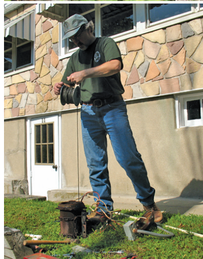
Figure 4, top , Mike Serfes points to a multilayered outcrop of slag associated with furnace smelting activities. Photo by S. Spayd . Figure 5, bottom , Steve Spayd using an M-scope to measure water level in a domestic well known to have high arsenic concentrations. Photo by T. Pallis
