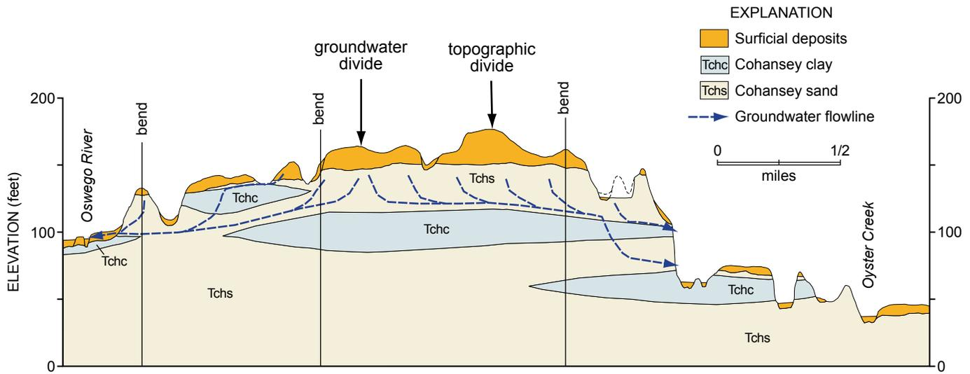
Figure 2. Cross section showing how lateral flow atop a clay bed diverts groundwater from the Oswego River basin into the Oyster Creek basin. Line of section shown in figure 3. Groundwater flow is shown schematically.
