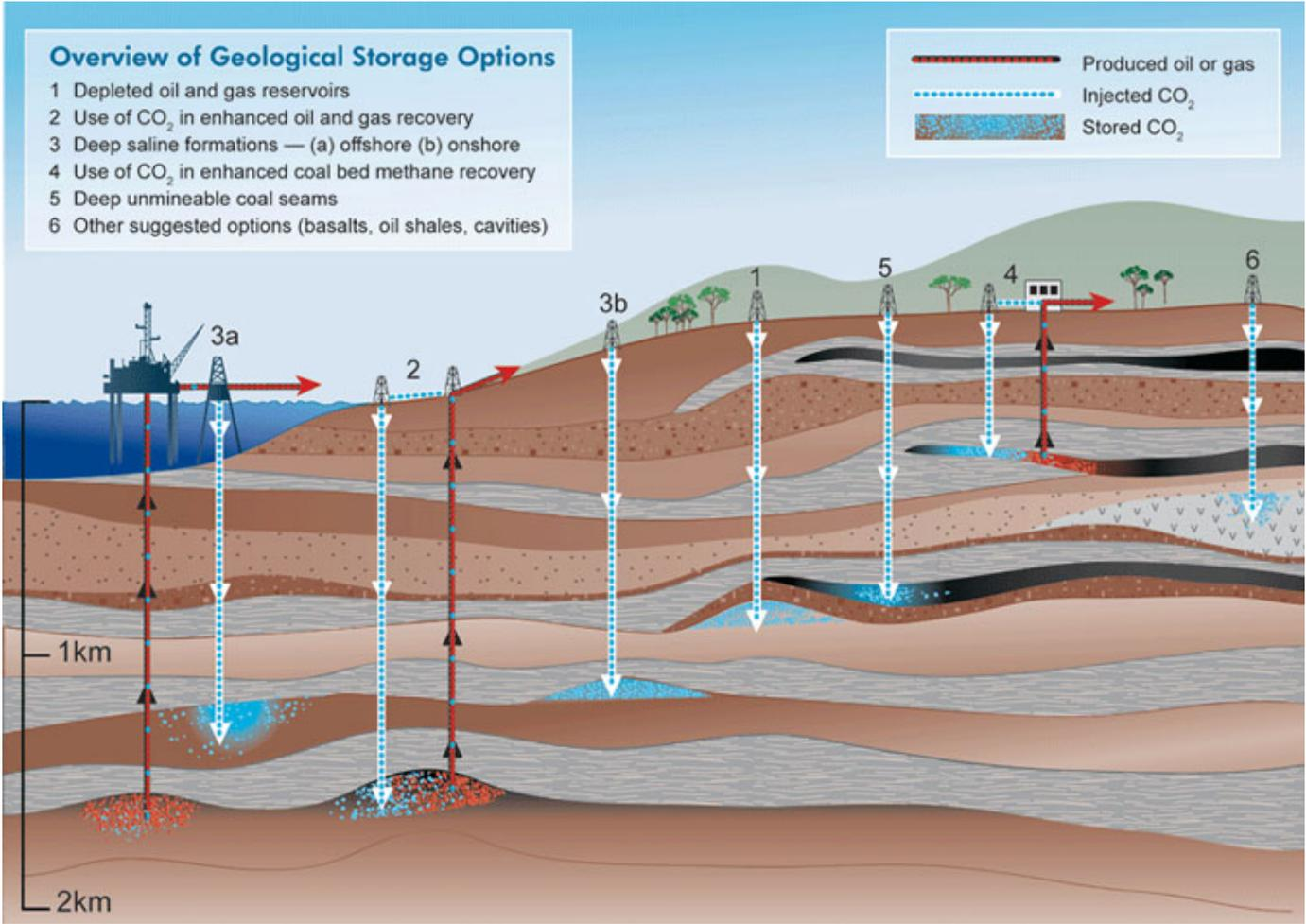
Figure 1. Types of CO<sub>2</sub> Geological Storage Options. In New Jersey, deep saline formations, both offshore (3a) and onshore (3b) offer the best potential for geological carbon sequestration. *Figure from [Intergovernmental Panel on Climate Change](#)*
