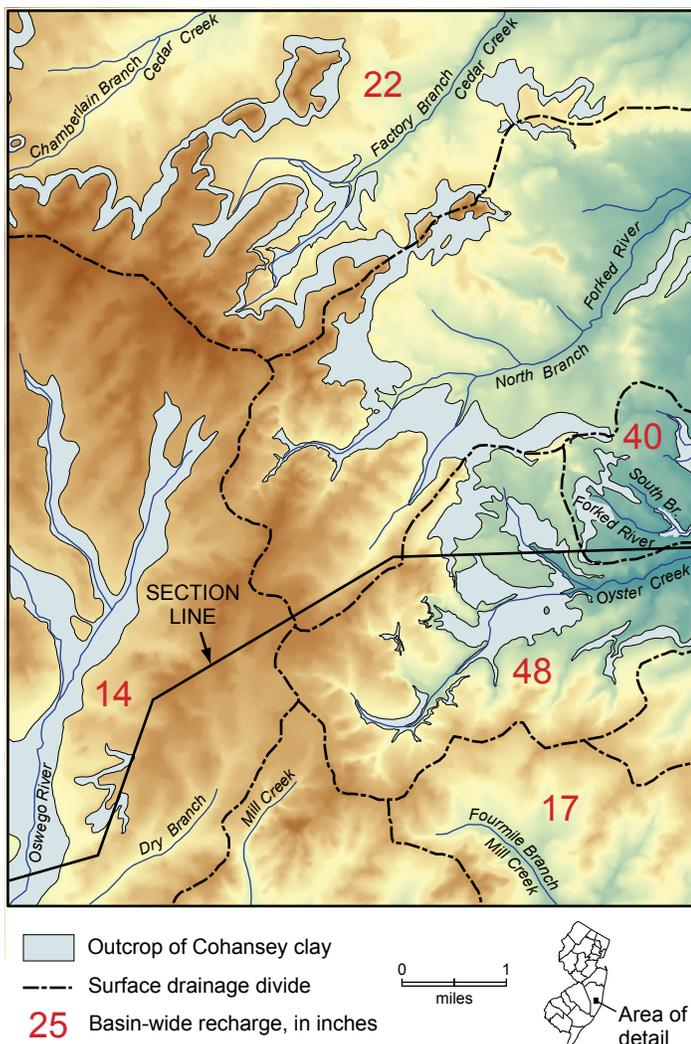
Figure 3. Outcrop of Cohansey clays in the Brookville quadrangle, and recharge rates for drainage basins showing eastward diversion of groundwater from the Oswego basin atop a clay bed. Elevation data from U.S. Geological Survey National Elevation Dataset, 10 meter resolution.
