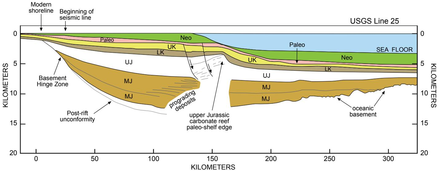
Figure 2. Schematic cross-sectional interpretation of USGS Line 25 based on Grow and others, (1988) and Poag (1985) across the New Jersey margin. LK (Lower Cretaceous) and UK (Upper Cretaceous) strata which are in part equivalent with the onshore Potomac Formation can be seen to thicken from onshore across the margin.
