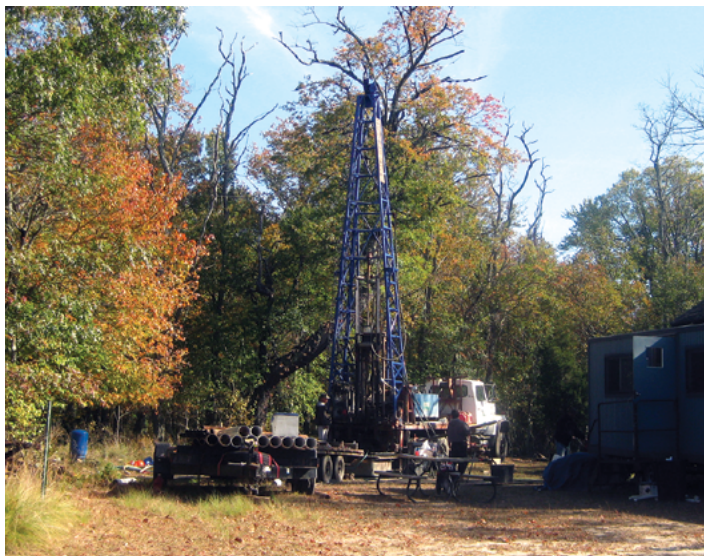
Figure 3. Double Trouble scientific coring site showing U.S. Geological Survey's Eastern Earth Surface Processes Team drill rig and scientific trailer. Photo by P.J. Sugarman
